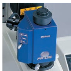
Focus pilot FP-05 Focus assisting system
