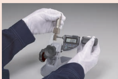
293-666-20 with fixing device 156-101-10 (optional accessories)
