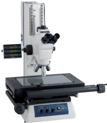
MF-UB 3017D (turret, objectives and illumination are optional)
