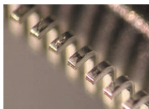
Measurement example : Height of leads on a QFP package
