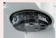
Power turret with 2 indenter mounts and 4 objective mounts
