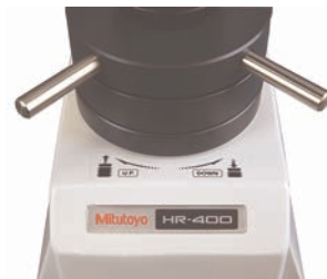
HR-400 Automatic preliminary test force brake
