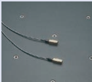
Temperature compensation system (temperature sensors)
