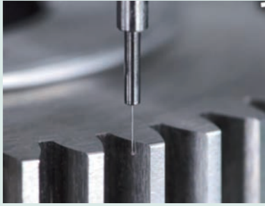
MPP-NANO Module 0.8 master gear measurement
