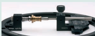
Holding a cylindrical part between clamping tips.
