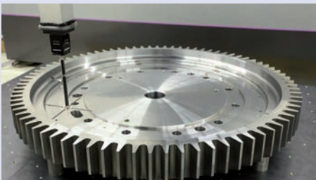
Scanning with probe SP80 and 100 mm styli.
