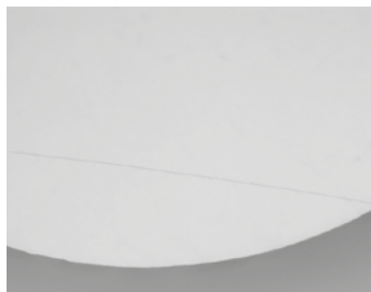
Scratched mirror-finished surface
