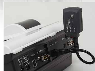
Example of SJ-310 installation
